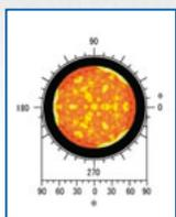
Experimental XPD photoelectron hologram of bulk 2s emission from Si(111) excited by Mg  $K_{\alpha}$  using a PHOIBOS 150 MCD-9 analyzer. The angular resolution was set with the Iris to  $1^{\circ}$  (data with courtesy of T. Matsushita, A. Agui and A. Yoshigoe, Spring-8, Japan)
