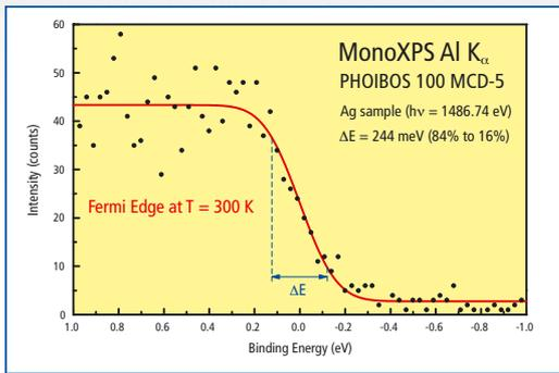
The spectrum shows the Fermi edge of Ag at 300 K measured with monochromated XPS. The width of the edge is 244 meV (84% to 16%).
