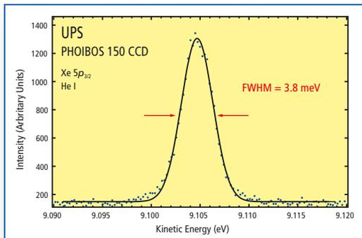
The Xe  $5p_{3/2}$  gas phase spectrum demonstrates the high energy resolution capability of the PHOIBOS hemispherical energy analyzer.
