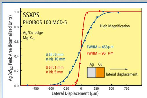
Small Spot XPS at a Ag/Cu edge with a broad illuminating source using the Iris aperture. The typical broadening of the acceptance area due to lens aberrations is eliminated.
