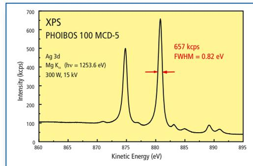
The intensity of the Ag  $3d_{5/2}$  photoelectron peak with a FWHM of 0.82 eV illustrates the resulting high count rate for a measurement with high energy resolution excited with non-monochromatized Mg  $K_{\alpha}$ .
