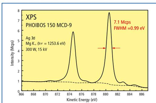
The Ag 3d peak obtained with the PHOIBOS 150 MCD-9 demonstrates the high étendue of the analyzer and the transfer lens.
