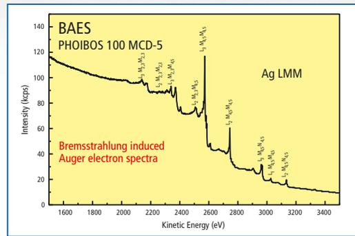
The advantage of BAES is a considerably improved signal-to-noise ratio compared to AES, because the background signal from inelastically scattered primary electrons is eliminated. This makes it unnecessary to differentiate the spectra.
