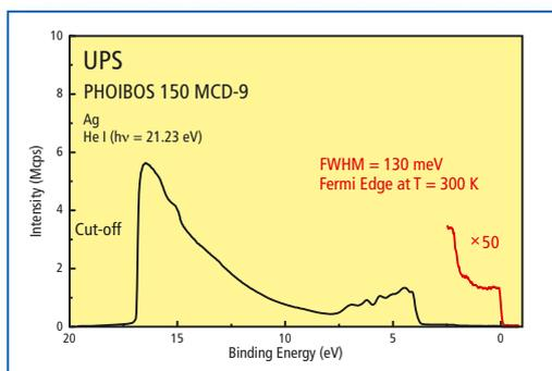
With the high brightness SPECS ultraviolet excitation sources the PHOIBOS analyzer series guarantees superior performance in ultraviolet photoelectron spectroscopy.
