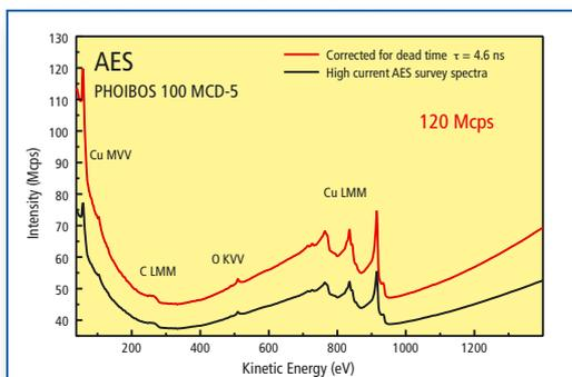
The high current AES survey spectrum shows the high count rate capability of the PHOIBOS detection system with the extended dynamic range CEMs.
