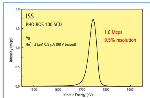
Ion scattering spectroscopy (ISS), performed with inverse polarity at the analyzer electrodes, is included in the standard package of analyzer and power supply.
