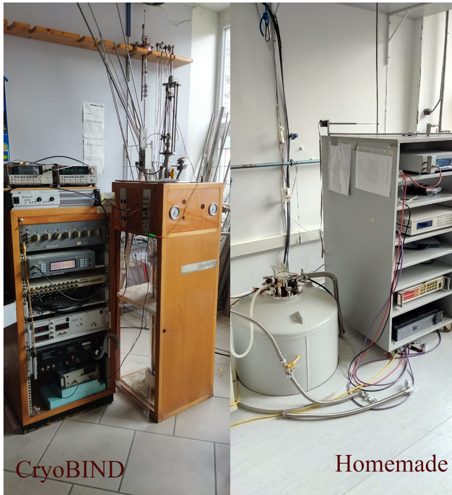
Figure 3.3: AC susceptibility measuring systems. Left is the CryoBIND, while right is the homemade system.
