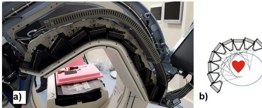
Figure 10. Detector configuration in Discovery NM 530c (a) and schematic representation of the detectors' field of view (b) [72].
